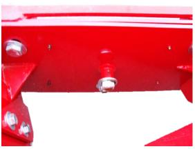
2 grease zerks on bearing at outer end of top auger. 4 pumps of grease every 4 hours of use.
