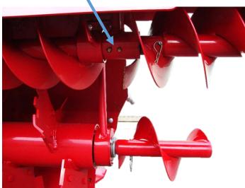
1 grease zerk on bearing at outer end of bottom auger. 4 pumps of grease every 4 hours of use.
