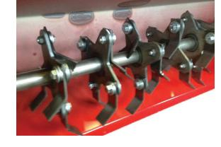
Can be replaced with latest style flail, hardened bushing, washer, and hardware.
